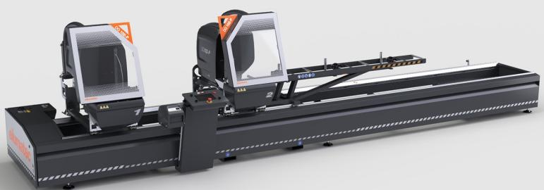
Electronic twin-head cutting-off machine with automatic traverse of the moving cutting head powered by brushless motor with numerical control system. Pneumatic control of the angular setting from 90° to 22°30' (external) in two fixed positions or with optional mechanic adjustment of intermediate angles. Hydro-pneumatic blade feed.
