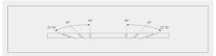
Mechanical adjustment of intermediate angles
